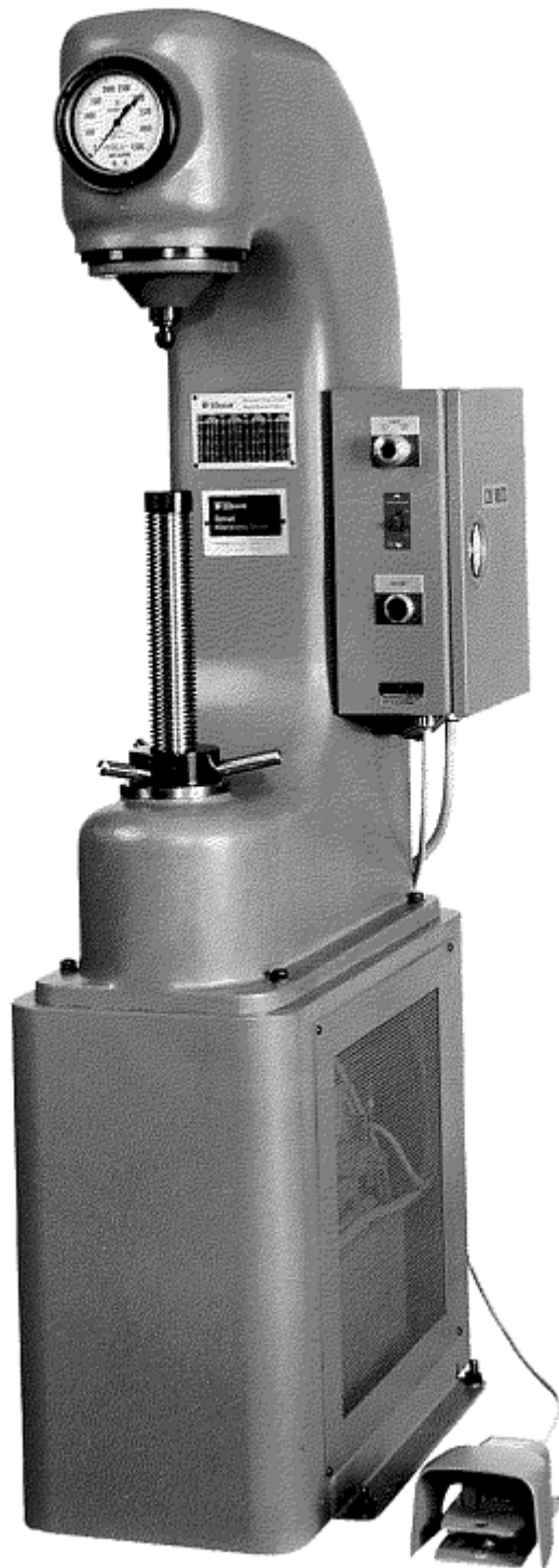
Fig. 16 Hydraulic Brinell tester. Courtesy of Wilson Instruments
