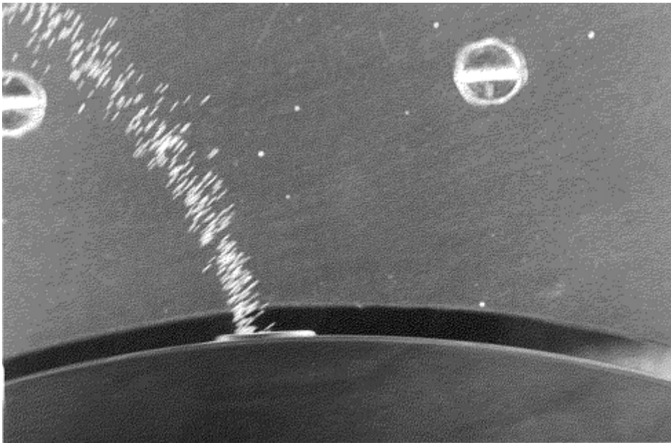
Fig. 8 Single flash exposure showing streak images of particle trajectories for olivine sand particles, 150–250 \mu\text{m} in diameter, leaving an acceleration tube at the rim of the rotating disk in a centrifugal accelerator of the design shown in Fig. 7. The disk was rotating clockwise and the mean particle velocity was 7 m/s. Courtesy of T. Deng and M.S.A. Bradley, University of Greenwich, UK
