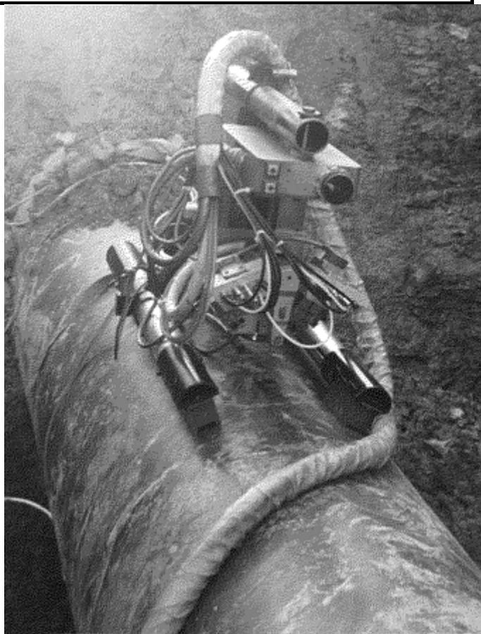
Fig. 1 Measurement of residual stresses on a gas pipeline in the field using a portable x-ray diffraction instrument. (Courtesy of Proto Manufacturing)
