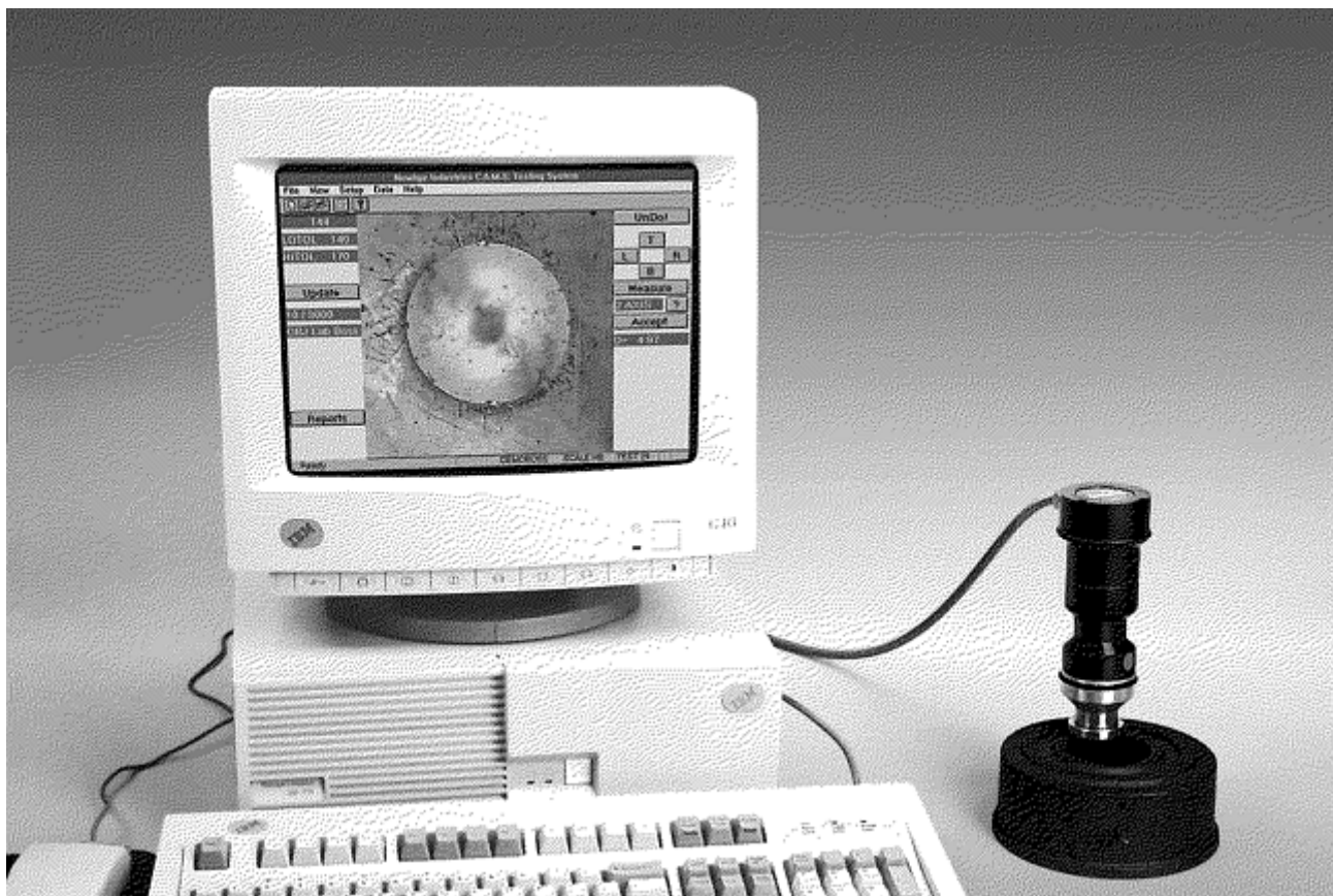
Fig. 14 Computerized Brinell hardness testing optical scanning system
