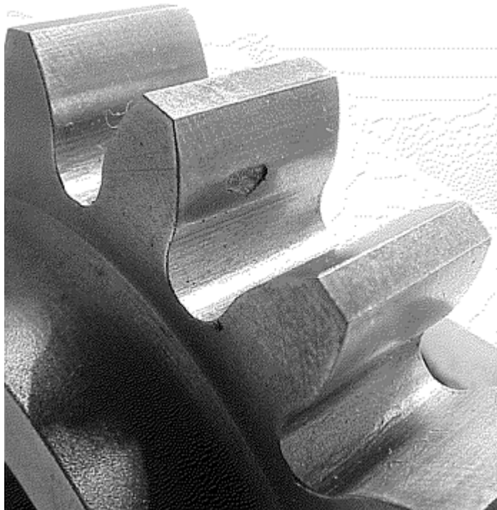
Fig. 4 Specimen gear with arrow-shaped surface origin pit
