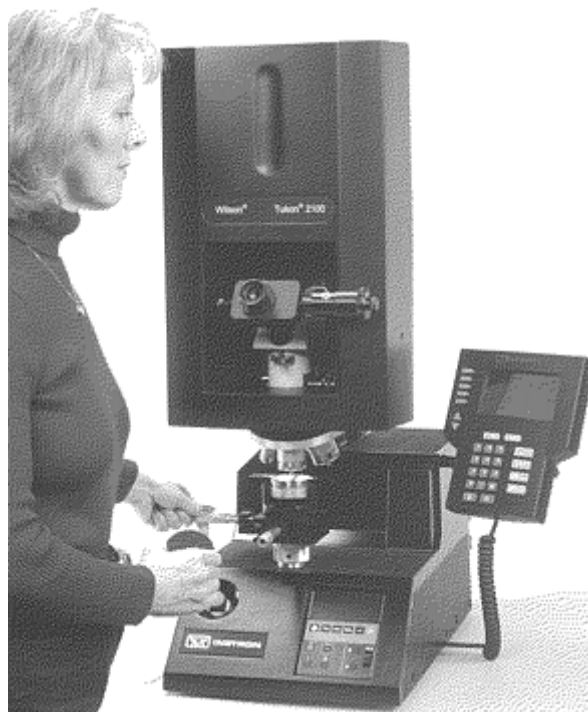
Fig. 5 Closed-loop load-cell microindentation hardness tester
