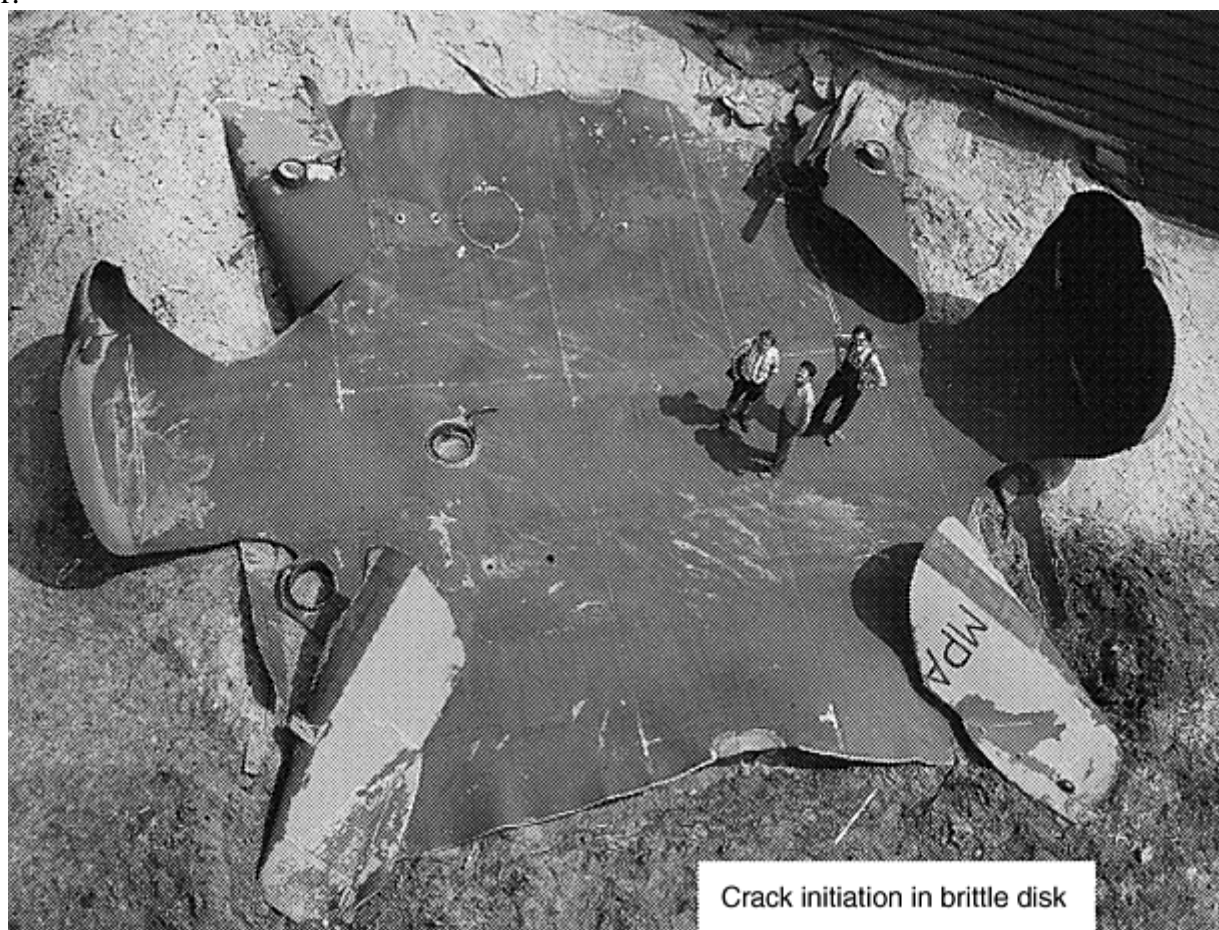
Fig. 20 Catastrophic failure at internal pressure of a feedwater tank
