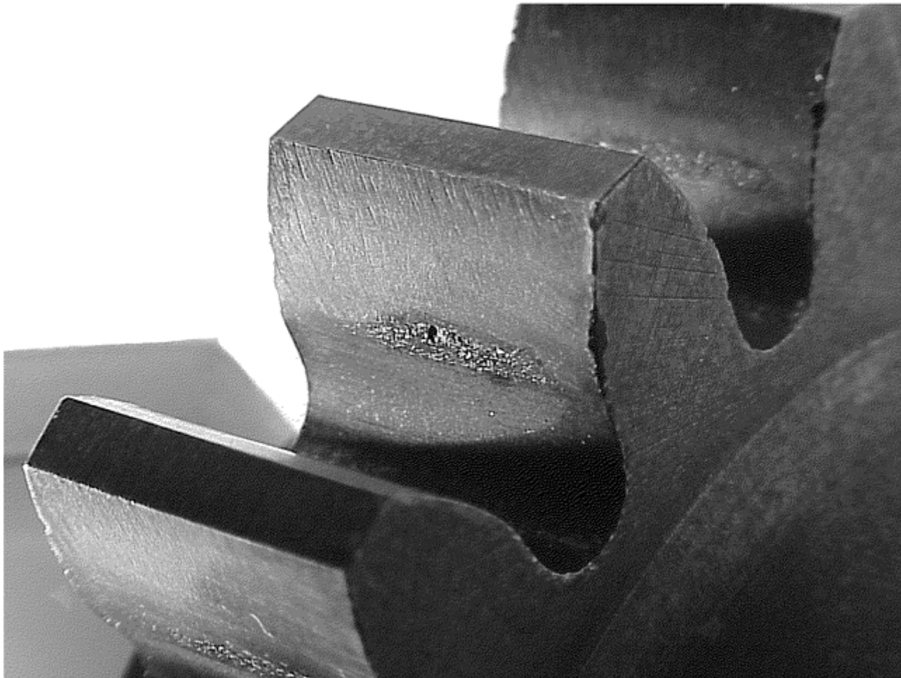
Fig. 3 Specimen gear with micropitting (frosting) failure
