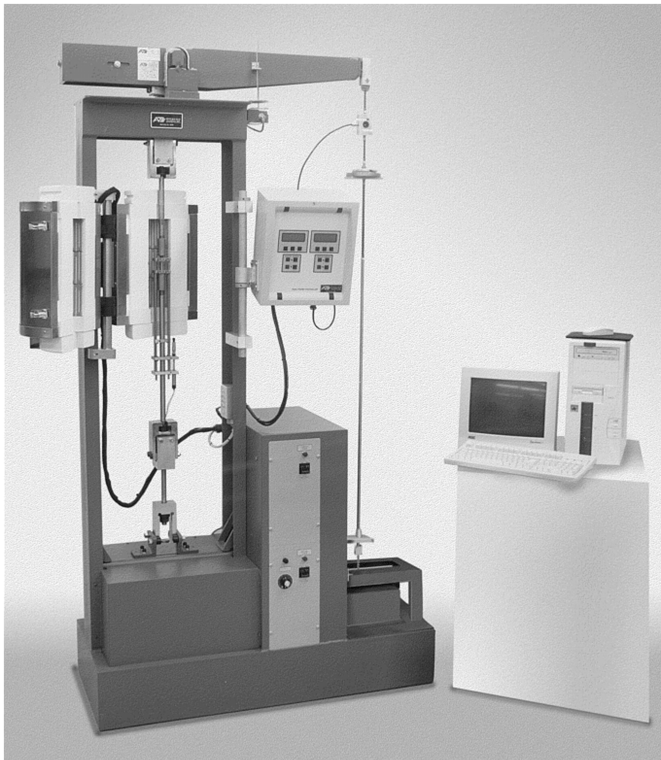
Fig. 18 Typical computer-controlled constant-stress test system with 90-kN (20,000 lbf) load capacity and furnace system.
