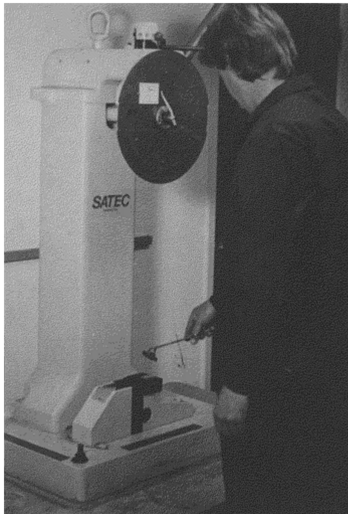
Fig. 8 Use of tongs to place a specimen in a Charpy impact testing machine for testing
