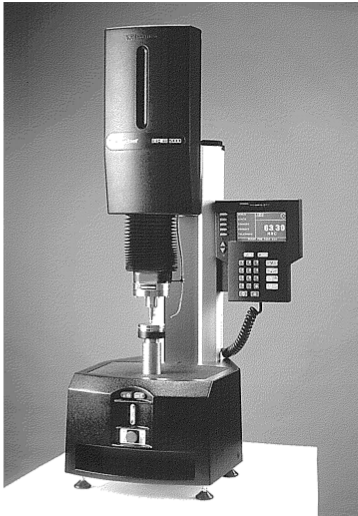
Fig. 4 Bench-type Rockwell tester
