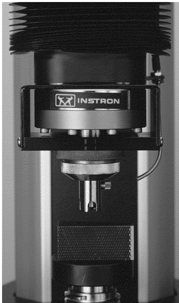
Fig. 8 Rockwell tester with removable clamping assembly
