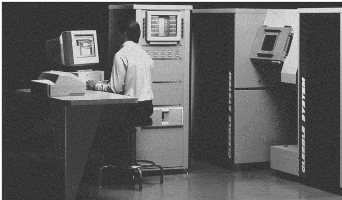
Fig. 26 A Gleeble 3800 testing system. Source: Ref 12
